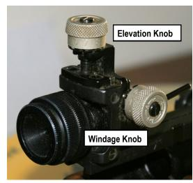
The knob on the top, the 'elevation knob', adjusts the sights vertically.
